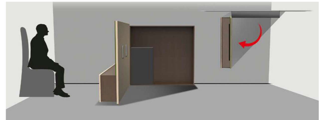
Figure 3.7 / Details of the technical compartment where all the home automation parts have been integrated and hidden from the end user.
