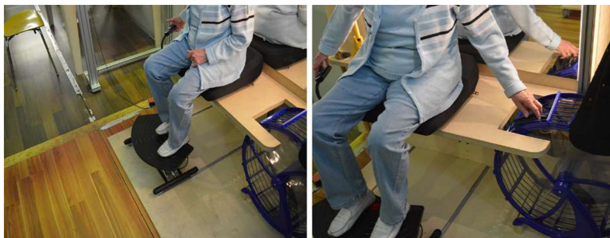
Figure 1.5 / Left: the moveable plate as support to put on shoes; Right: the ergonomic shoe shelf.
