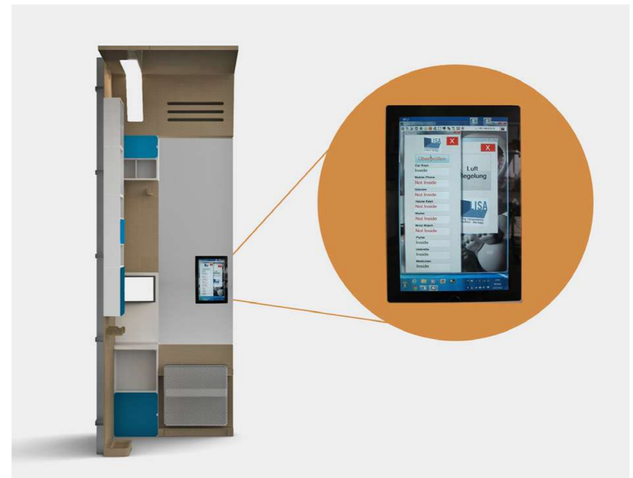
Figure 1.11 / GUI on the touch screen as user interface; showing the result of the RFID tag scan.
