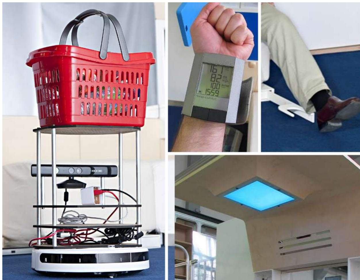
Figure 1.7 / Prototype service modules for the smart AAL walls. Bottom right is light and air purifier. Left is a robotic assistance. Top right is a shoehorn for assistance with putting on shoes. Top middle is the blood pressure meter for health status estimation.
