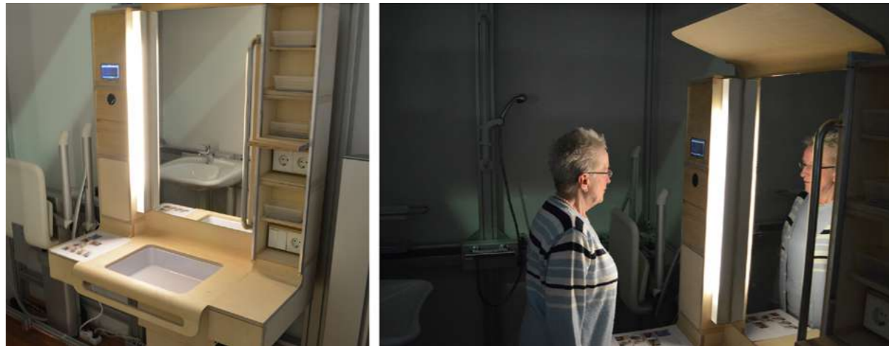
Figure 2.7 / Left: the bath terminal module. Right: testing the fever detection.
